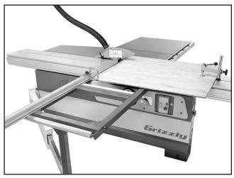
Figure 50. Rip cutting with the sliding table.
